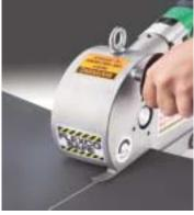
The Electric Belt Cutter is available in two sizes and specifically designed to allow the end user to cut belts quickly and safely resulting in less conveyor downtime, and overall increased productivity. The EBC1 Electric Belt Cutter is capable of cutting a rubber belt up to 1" (25 mm) and up to a maximum 360 P.I.W. (630 N/m) on PVC belts while the EBC2 cuts rubber belts up to 2" (50 mm) and up to a maximum 1140 P.I.W. (2000 N/m) on PVC
